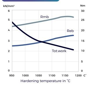
Original dimension Ø 6 mm Tempering 3 x 1 hour at 560°C Dimension of test piece Ø 4.7 mm
