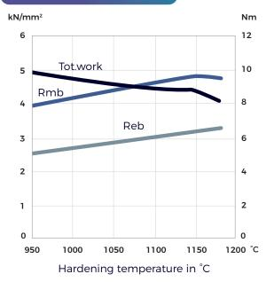
Original dimension Ø 16 mm Tempering 3 x 1 hour at 560°C Dimension of test piece Ø 4.7 mm
