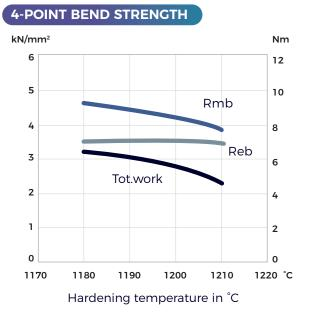
Original dimension Ø 5.6 mm Tempering 4 x 1 hour at 560°C Dimension of test piece Ø 4.7 mm
