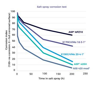
Corrosion resistance from salt spray test of different types of Powder Metallurgy martensitic steels tempered  $< 300^{\circ}$ C.
