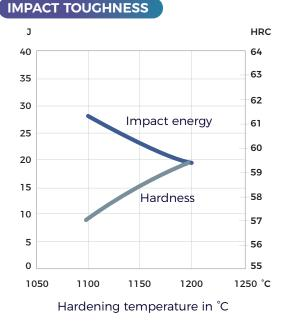
Original dimension 260 x 174 mm Tempering 2 x 2 hours at 540° C Unnotched test piece 7 x 10 x 55 mm
