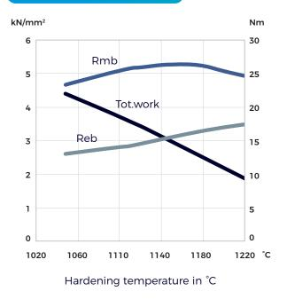
Tempering 2 x 1 hour at  $560^{\circ}$ C Dimension of test piece Ø 4.7 mm
