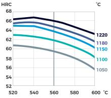
Tempering temperature in °C Hardness after hardening, quenching and tempering 2 x 1 hour
