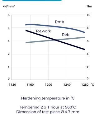
Rmb = Ultimate bend strength in kN/mm<sup>2</sup> Reb = Bend yield strength in kN/mm<sup>2</sup> Tot. work = Total work in Nm
